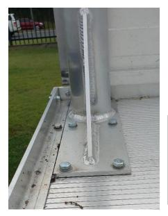
Left, Factory Hino and Triple M trays: Sharp 30mm edge angle. This off-the-shelf extrusion serves no purpose, locks in dirt and damages cartons when sliding over. Lifting items over can cause injury to driver
